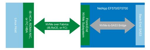
Figure 3) NVMe front end on EF570 and E5700 systems.
