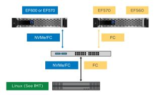
Figure 6) Coexistence between NVMe/FC and FC.
