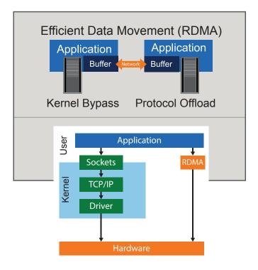
Figure 1) RDMA with Mellanox ConnectX InfiniBand Adapters.
