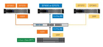
Figure 4) Coexistence between NVMe/IB, iSER, and SRP.
