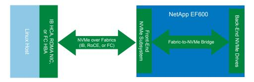
Figure 2) NVMe end to end on an EF600 system.
