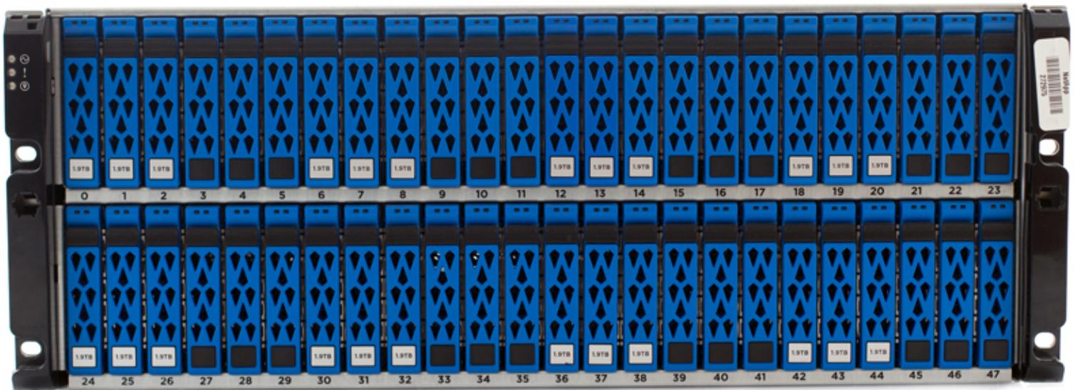
Looking at the NVMe drives themselves, NetApp supports a wide range of capacity options including 1.9TB, 3.8TB, 7.6TB and 15.3TB SSDs. As of this writing, NetApp is shipping all of these drives as self-encrypting (SED) with AES-256 encryption. Additionally, for systems initialized with ONTAP 9.4, fast drive zeroing is enabled.
