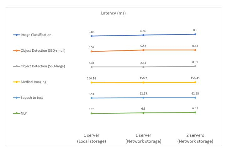
The results, again, show that the network storage is sufficient to handle the tasks. The difference between local and network storage in the one server case is minimal or none. Similarly, when two servers use the same storage, the latency on both servers stays the same or changes by a very small amount.
