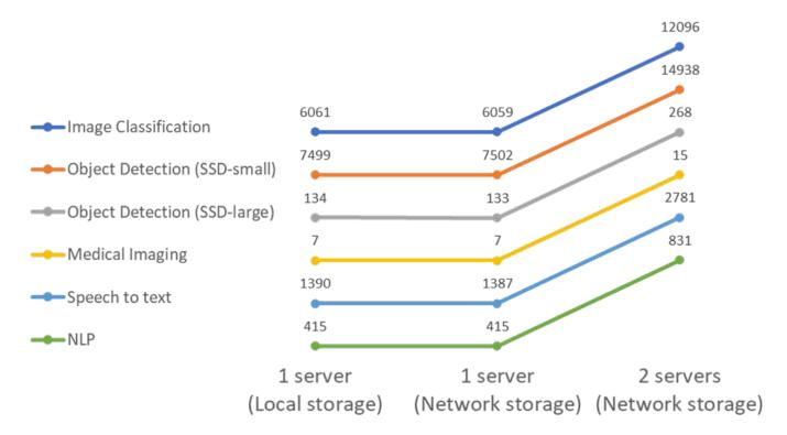
The results show that network storage does not negatively affect the performance—the change is minimal and for some tasks, none is found. When adding the second server, the total bandwidth either exactly doubles, or at worst, the change is less than 1%.
