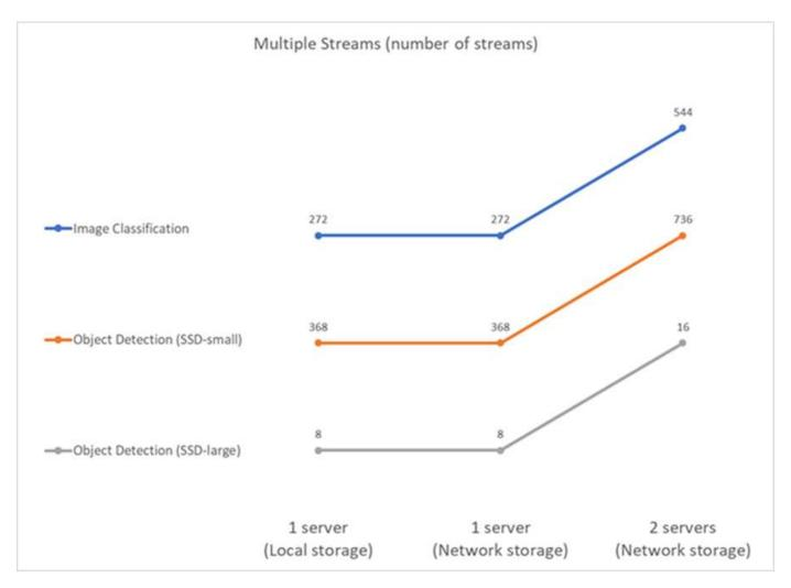
The results show perfect performance of the setup—local and networking storage give the same results and adding the second server doubles the number of streams the proposed setup can handle.
