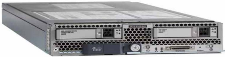
Figure 7. Cisco UCS B200 M5 Blade Server front view
